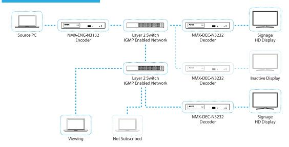
If the AV network will span multiple subnets or VLANs, a second control can be implemented. PIM (Protocol Independent Multicast) allows for the sending of multicast across any subnet and/or VLAN where PIM is enabled. In these scenarios, additional network devices may be needed to facilitate this functionality.
